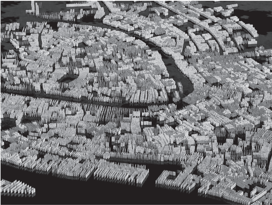
In the images: Axonometric view of the 'muri di spina' walls of Venice
